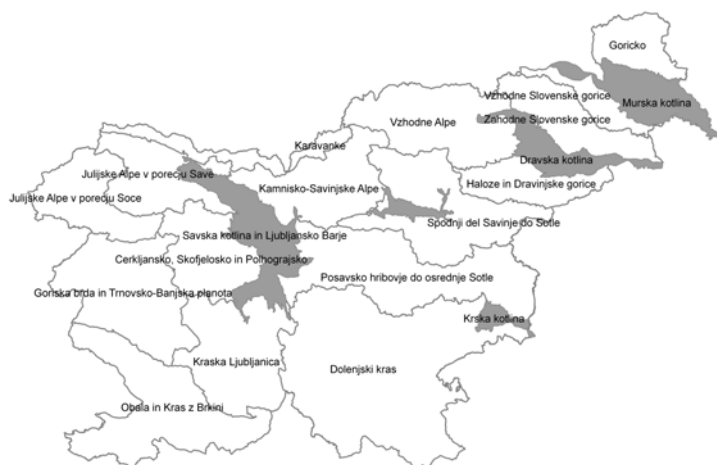
Figure 1: Groundwater bodies in Slovenia according to the prevailing porosity of the aquifers. Groundwater bodies with aquifers with prevailing intergranular porosity are shaded. Non shaded are groundwater bodies with aquifers with prevailing karst, fracture and mixed porosity [3]
