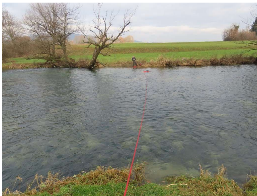
Slika 1. Meritve pretoka Krke v njenem povirju na območju Podbukovja, 17. decembra 2020 (foto: arhiv ARSO) Figure 1. Krka river discharge measurement on 17 th of December 2020 at its headwaters in Podbukovje (photo: ARSO archive)
