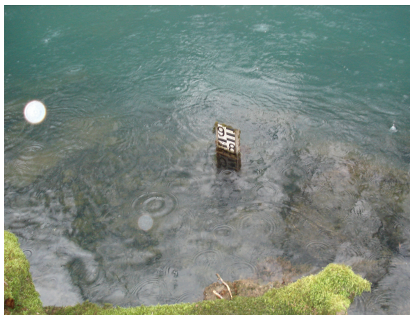
Slika 2. Vodometna lata na merilnem mestu Krupa - Dolence I (foto: Marko Rus) Figure 2. Gauge at gauging station Krupa – Dolence I (photo: Marko Rus)
