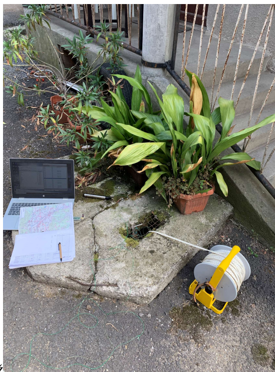
Slika 2. Izvajanje kontrolne meritve in prenosa podatkov višine gladin podzemne vode, julij 2021 Figure 2. Control measurement and groundwater level data transmission performance, July 2021
